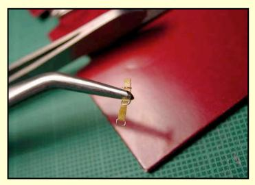
Poke a piece of the fuse wire through the fold and flatten the tape down again. You have to do this very gently or you'll distort the wire link.
